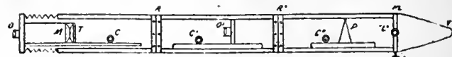
O, O', lenses; M, single lenses; T, screen; C, C', rack and pinions; R, R', hinges; P, prism; Pl, plate; L, L', micrometric screws; V, eye-hole.
